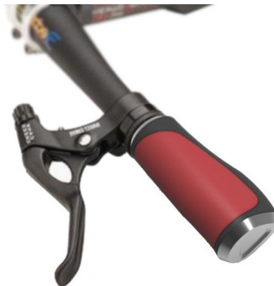
Figure.6 The trapezoidal block of Rush material was designed in accordance with the fingers grip to increase comfort.
