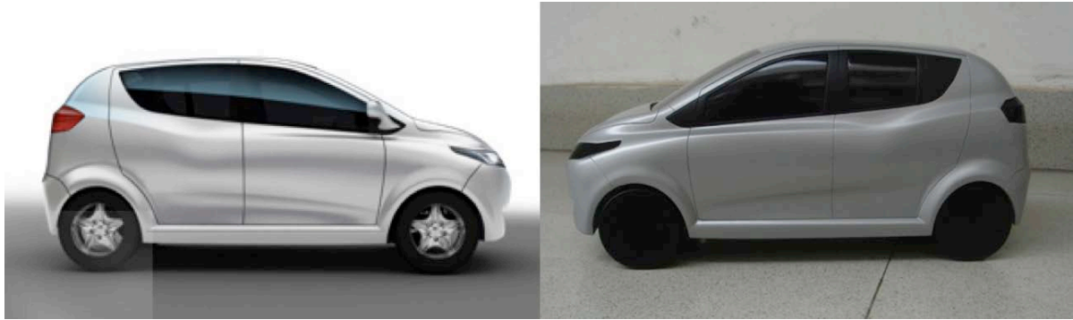
Figure 9. The expression and 1:10 model of new Changan Benben designing based on the feature lines
