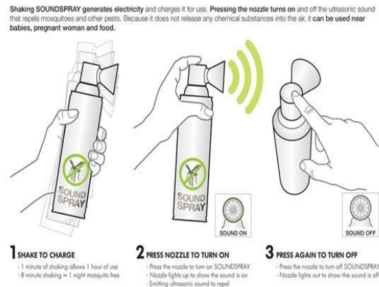
Figure.2 How Soundspray works
