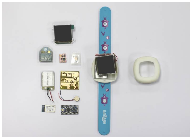
Figure 15. Wearable prototype for in-situ user testing
