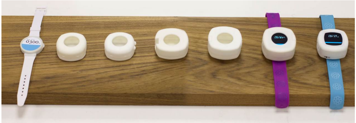
Figure 14. Exploration of the casing for the watch module
