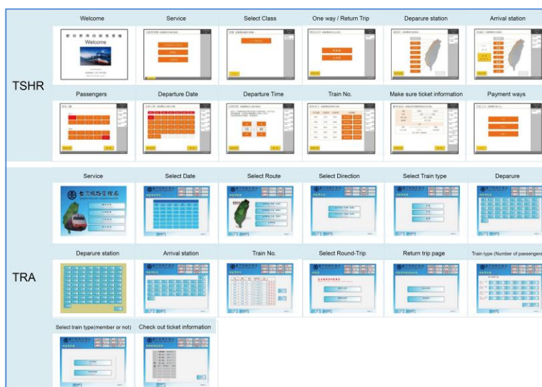
Figure.2 The various operation sequence of existing ticket vending machine systems frequently confused the passengers (upper: TSHA and lower: TRA).
