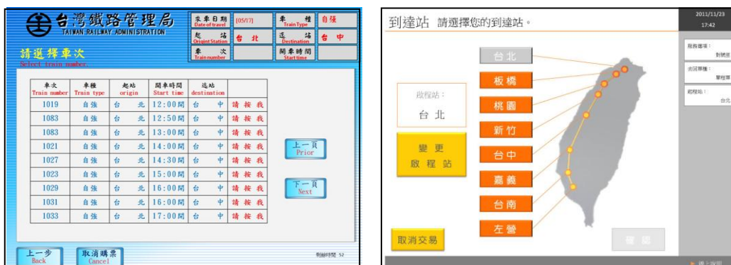
Figure.3 Existing ticket vending machine systems in layout fundamentals such as shape, size and position of option buttons in TRA and TSHA need to be redesign employing the principle of interface consistency, overview plus detail (OPD) and metaphoric interfaces
