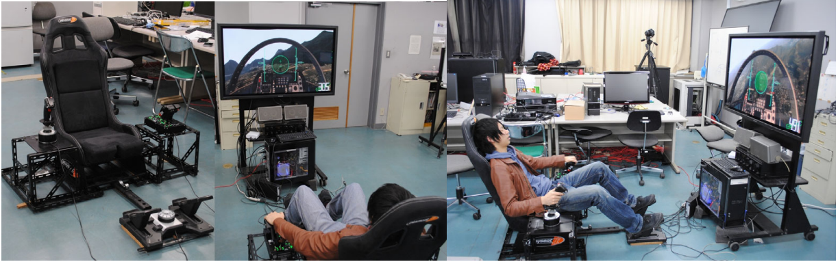
Figure 4. A prototype of physical user interface of air-craft.
