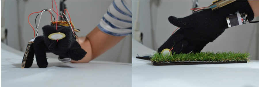
Figure 4. Glove sound generator. Sound is generated by touching and stroking different textures.
