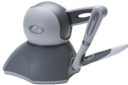
Figure.3 Photo of the Phantom Omni haptic feedback device from Sensable, used with permission by Sensable Technologies Inc.
