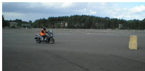
Figure 3. Live testing of PTW impacting a stationary object
